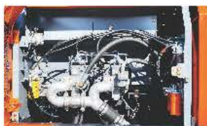
Grouped remote filters and inspection points
