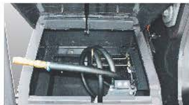
Electric fuel refilling pump
