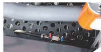
Fuel tank water drainage cock
